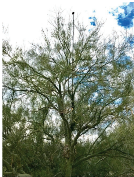
An example of cryptic placement of bat acoustic monitoring equipment. Credit Jessie Dwyer.
