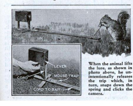
AN ORDINARY mouse trap and a few feet of <sup>1</sup>/<sub>2</sub>"x1<sup>1</sup>/<sub>4</sub>" stock are all the parts required to make this automatic shutter release for your box camera. The device, which should be painted green, is unique in catching unusual poses of small forms of wild life.
